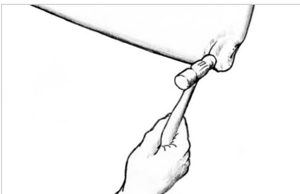
Figure 8-2 Use a ball-peen hammer, with repeated light taps to work the lead bulge back to its original shape.
