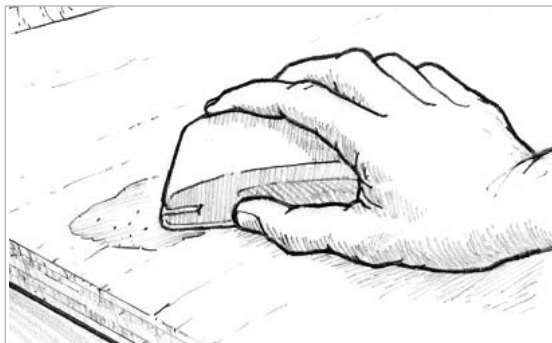
Figure 9-16 Sand the fairing material to blend with the surrounding contour.
