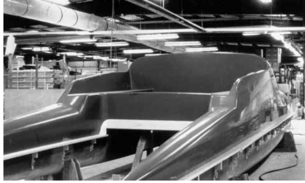
Figure 3-3 The catamaran plug was faired and finished to the same degree as the finished product. The shelf was applied to the plug where the mold halves divide the form at its widest point.
