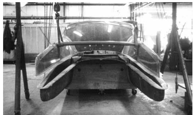
Figure 4-7 A finished laminated part (deck/cabin), suspended over the bottom (hull) mold. The mold also serves as a jig to hold the laminated hull in while interior components and the laminated deck are bonded in place.
