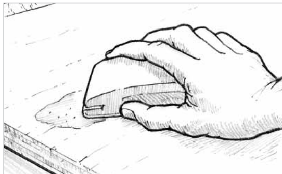
Figure 5-16 Sand the fairing material to blend with the surrounding contour.
