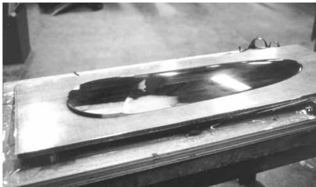
Figure 3-4 A plug for a rudder, with the shelf positioned at the rudder centerline, is waxed and ready for the application of the mold half.
