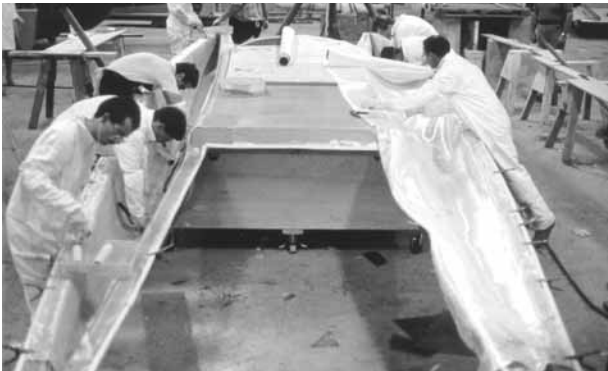
Figure 4-2 Fiberglass cloth is wet out in the bottom (hull) mold of the 32' catamaran after the cured epoxy gelcoat is washed and sanded.
