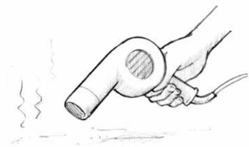
Figure 7 Dry the surface. Allow wet surfaces to dry thoroughly or use heat or a fan to speed drying.
